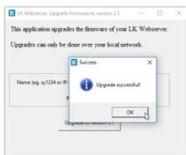
If the upgrade fails check the ID and password and try again or use the IP address instead of the Webserver ID to login.
