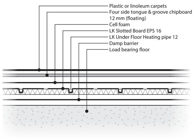
LK EPS 16 laid out "floating" on load bearing floor in dry areas. Surface layer plastic or linoleum carpets
