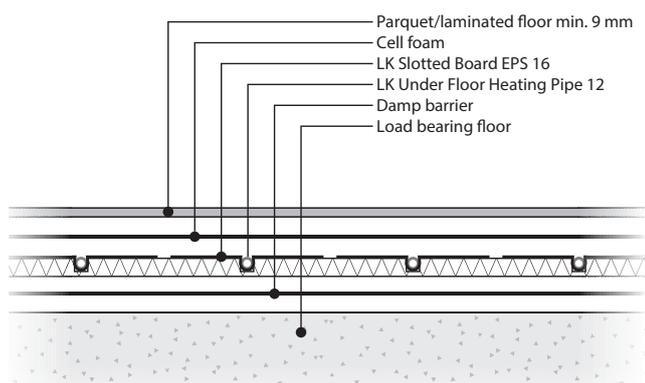
LK EPS 16 laid out "floating" on load bearing floor. Surface layer parquet.
