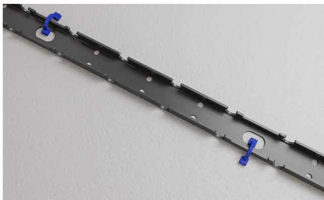
Alternate the clips' attachment from side to side over the clip rail for best stability. Use 3 pcs clips per clip rail of 2 m length and use 4 pcs clips for clip rail with 4 m length.
