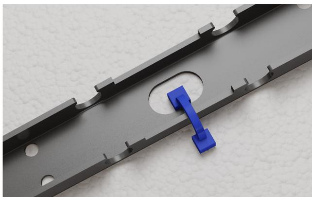
In order to fix LK Clip rail 16 the staple is pressed over one edge of the rail. The clip will then attach through the pressed oblong attachment hole in the rail's base and outside rail.
