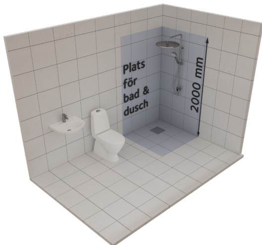
Wet zone 1 for showers.
