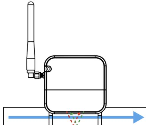
The CubicMeter measures the flow of water with the use of ultrasonic waves and the “differential time of flight” method. To measure the flow of the water, two ultrasonic transducers transmit signals in opposing directions through the pipe and water as illustrated in the above image.
