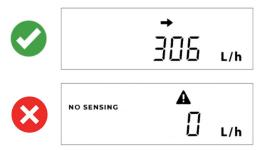
6. If the "no detection" symbol is displayed, verify steps 1-4 or try a different mounting position/rotation of the pipe.
