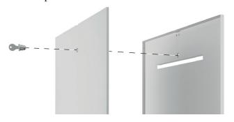
5. Insert the lock nut and locking plate at the back of the hatch. Put the parts together and tighten the lock nut.
