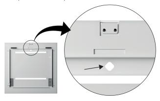
2. Use the hole in the hatch for the locking bolt as a template. Drill a hole in the plasterboard for the locking bolt.
