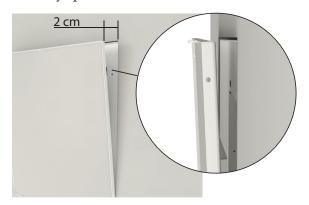
2. Get a good grip with both hands on the sides of the hatch and lift it carefully upwards. Adjust the lifting until the pins disengage and the hatch is released.
