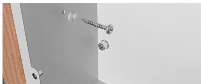
Attaching a cabinet to a stud wall.
