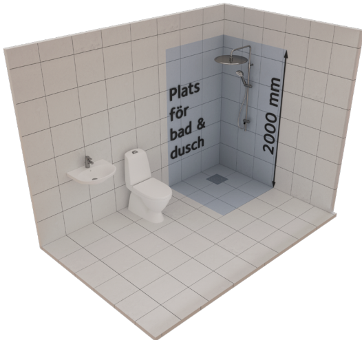
Wet zone 1 for showers.
