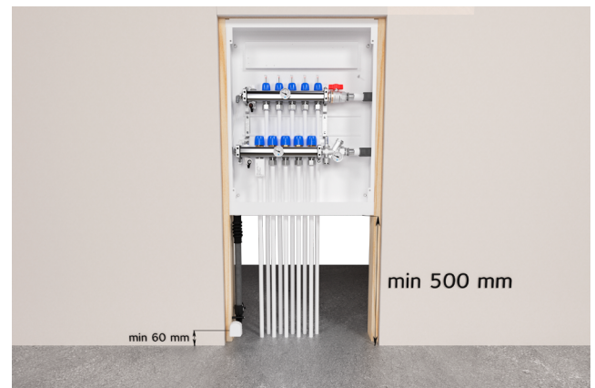
Picture of fitting a cabinet 500 mm from floor surface.
