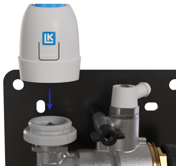
Step 4: Mount the actuator on the gray adapter. A click is heard when the adapter is installed correctly.
