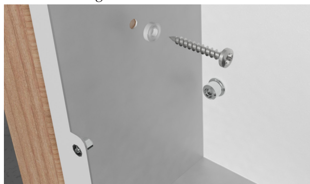
Securing the cabinet in a stud-frame
