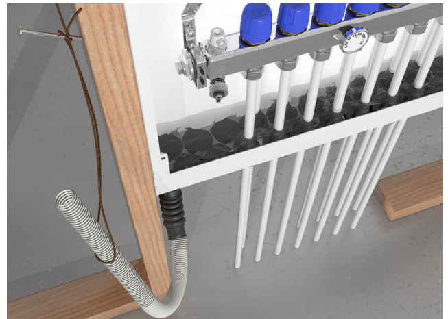
Principle diagram for leak testing of the cabinet base
