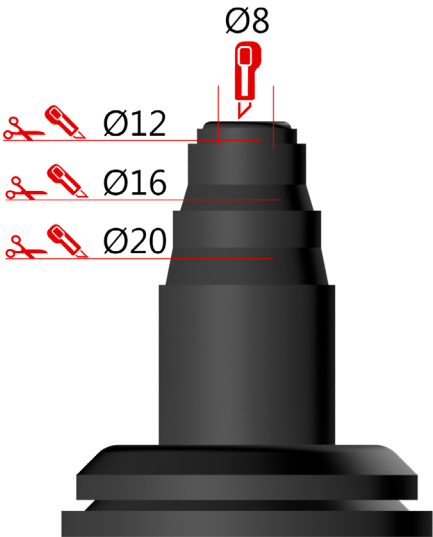
Cutting of pipe grommet.
