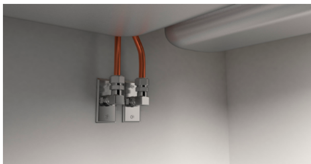
When penetrations for LK PE-X and PAL Universal pipes Pipe-in-Pipe without a wall box are to connect to a kitchen or washbasin mixer, for example, the angle at the transition between the LK PE-X – LK PAL pipe and the mixer’s connecting pipe must be fixed. This is preferably done using a wall washer fitted with thread connection.
