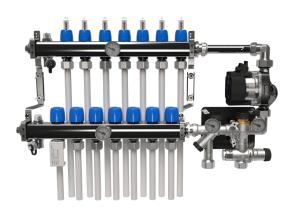
The shunt unit can be mounted directly to LK Manifolds from both the right and left. To facilitate this, two Manifold Supply Pipes are supplied, where the shorter is used for right mounting, see illustration above.
