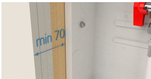
At least 70 mm from the outside plaster to the front edge of the cabinet
