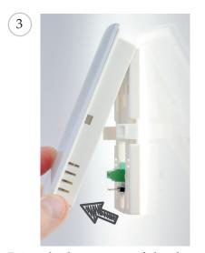
Bring the lower part of the thermostat outwards from the wall.
