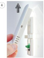
Bring the thermostat straight upwards along the wall.
