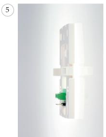
The thermostat is separated from the wall mount. The wiring and connectors are intact. This means that the wall mount doesn't need to be replaced.
