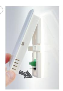
Push the lower part of the thermostat towards the wall mount. Take care not to damage the connection pins on the wall mount when remounting the thermostat.
