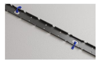
Alternate the clips' attachment from side to side over the clip rail for best stability. Use 3 pcs clips per clip rail of 2 m length and use 4 pcs clips for clip rail with 4 m length.
