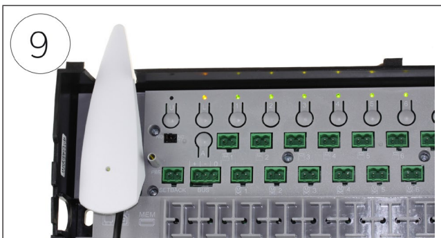
The receiver unit's L-LED switches to yellow and selectable channels light up green. Select channel by pressing desired channel key. The selected channel flashes green.
