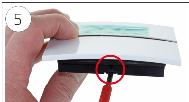
5 Remove the back of the thermostat by pressing the locking with a screwdriver or similar.
