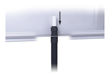
• Slide the LK Umbrella LP seal over the inner pipe and down over the rubber inlet.
