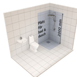
No service opening must be positioned in places for a bath or shower.
