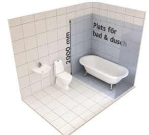
No service opening must be positioned in places for a bath or shower.
