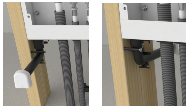
A drainage elbow directly connected to the cabinet's outlet pipe will drain into the same room as the cabinet's service hatch or, alternatively, the room behind.
