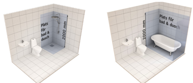
No service opening must be positioned in places for a bath or shower.
