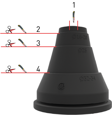
Cutting LK Pipe lead-through 20-25 LP.
