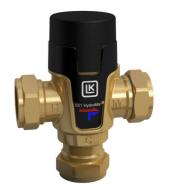
When fitted on top of boiler/storage tanks with built-in water heaters the valve should be installed with some space between boiler/storage tank and valve so as not to let the function of the valve be affected by heat radiation.
