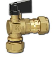
Installation of the compression fitting is facilitated if lubricant is applied to the thread and chamfer. Tighten manually as far as possible, then use a fixed wrench. Tightening, number of turns with wrench plus other technical data - see separate data sheet for compression fittings. Soft pipes are fitted with support sleeves. The valve requires no maintenance. The installation should be checked regularly.
