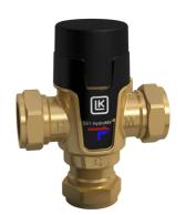
When fitted on top of boiler/storage tanks with built-in water heaters the valve should be installed with some space between boiler/storage tank and valve so as not to let the function of the valve be affected by heat radiation.
