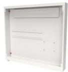
The cabinet has a dense base with rubber pipe grommets. The cabinet base is provided with a drainage opening which allows any water leakage to be drained to a location which can be inspected. The cabinet is manufactured from 1 mm powder-coated sheet steel, RAL 9016.
