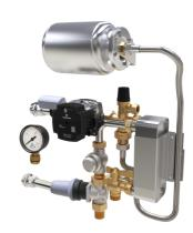
For weather compensated heat regulation for floor heating LK Heat Exchanger Pack can be equipped with LK Control v.3- RA. LK Control v.3-RA consists of a control unit, valve actuator, outdoor sensor and supply temperature sensor.
