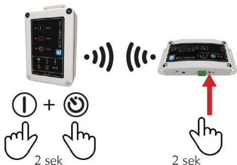
Programming the leakage detector.
