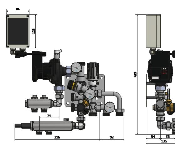
LK Heater for a single floor heating circuit assembled with LK Minshunt M60n.
