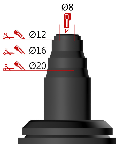
Cutting of pipe grommet.
