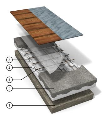
House foundation slab shall be designed taking into account the load of the house in accordance with EN 206-1. A "rule of thumb" for a normal house with a so-called slab on ground is that the concrete strength class must be at least C20/25.
