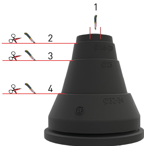
Cutting of a LK Pipe Inlet 20-25 LP.
