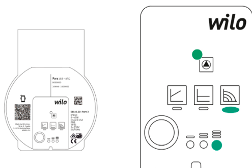
Wilo Para 25-130 / 6-43 SC with factory-set display.
