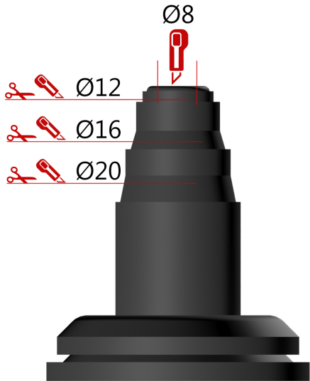
Cutting of pipe grommet.
