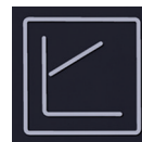
The symbol for proportional pressure.
