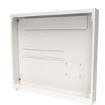
The cabinet is designed for installation built into a wall or surface-mounted on a wall. When building in the cabinet, the minimum stud thickness is 95 mm. The cabinet must be supplemented with a frame/hatch. There are two types of frame/hatch, depending on whether the cabinet is built into or surface-mounted on an inner wall. When surface-mounted, the cabinet must also be supplemented with a base in order to conceal pipes between the cabinet and the floor.
