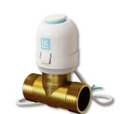
LK Thermostat Valve Kit is used for the individual control of respective floor heating circuit on the LK Mini Manifold. The assembly kit includes a LK Thermostat Valve Mini  $\frac{1}{2}$ ", a LK Actuator 24V NO, nipple connection  $\frac{1}{2}$ " for the Mini Manifold 12 or 16, as well as a pipe connection coupling 12 or 16.
