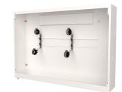
The cabinet is manufactured from 1 mm powder-coated sheet steel, RAL 9016. The cabinet is designed for installation built into a wall or surface-mounted on a wall. When building in the cabinet, the minimum stud thickness is 95 mm. The cabinet should be assembled according to the industry regulations "Säker Vatteninstallation".
