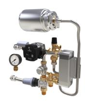
For weather compensated heat regulation for floor heating LK Heat Exchanger Pack can be equipped with LK Control v.3- RA. LK Control v.3-RA consists of a control unit, valve actuator, outdoor sensor and supply temperature sensor.
