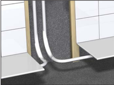
Figure 7. Installation of an LK Pipe Bending Support.
